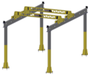
4 Overhead 20 Ton Cranes
